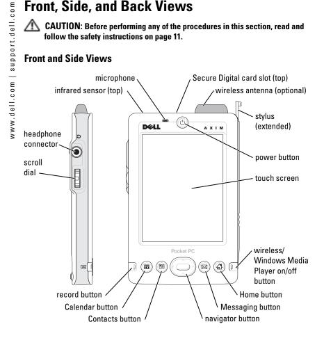
INFRARED SENSOR—The infrared sensor lets you transfer files from your device to another infrared-compatible device without using cable connections.
